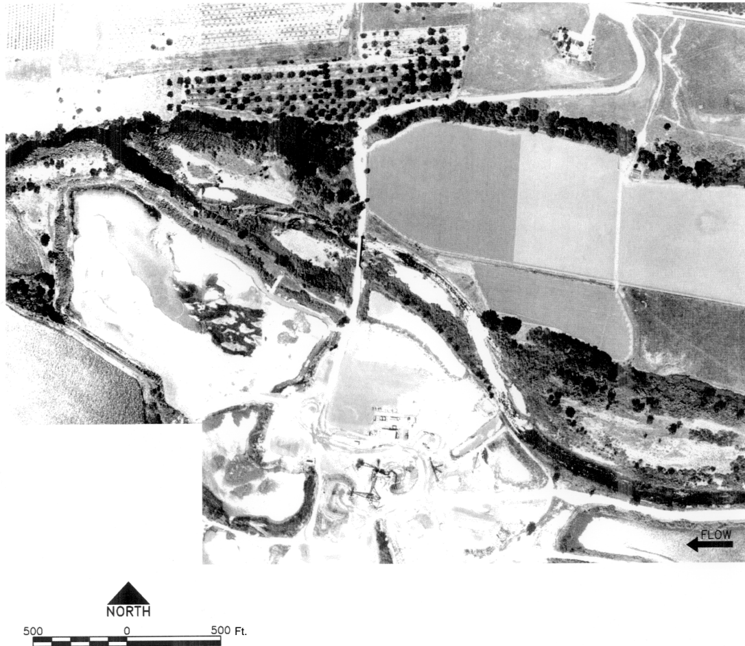
Figure 2-21. 1993 example alternate bar sequence in gravel-bedded reach, near 7/11 Materials plant site at RM 38, showing aggregate extraction on historic floodplain surfaces and confinement of contemporary floodway with dikes and encroached riparian vegetation. Compare to Figure 2-19.
